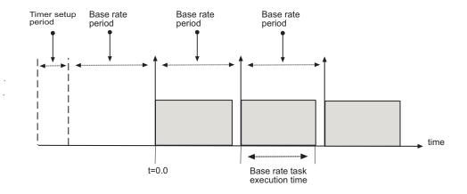
Timer-based scheduling does not provide enough flexibility for some systems. Systems for control and communications must respond to asynchronous events in real time. Such systems may need to handle a variety of hardware interrupts in an asynchronous, or *aperiodic*, fashion.
