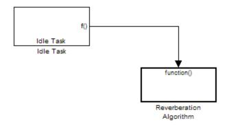
The function generated for this task normally runs in free-running mode—repetitively and indefinitely. Subsystem execution of the reverberation function is data driven via a background DMA interrupt-controlled ISR, shown in the following figure.
